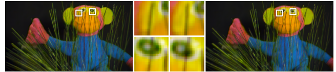
Figure 11: Reconstruction of a partly-occluded scene. Two views of a light field reconstructed from a single camera image. Areas occluded by high-frequency structures can be recovered by the proposed methods, as seen in the close-ups.
