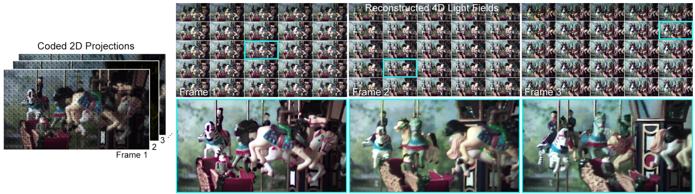
Figure 12: Light field reconstructions of an animated scene. We capture a coded sensor image for multiple frames of a rotating carousel (left) and reconstruct 4D light fields for each of them. The techniques explored in this paper allow for higher-resolution light field acquisition than previous single-shot approaches.
